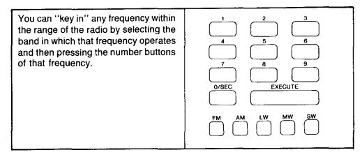
Example: To tune to 7305 kHz on the AM band
